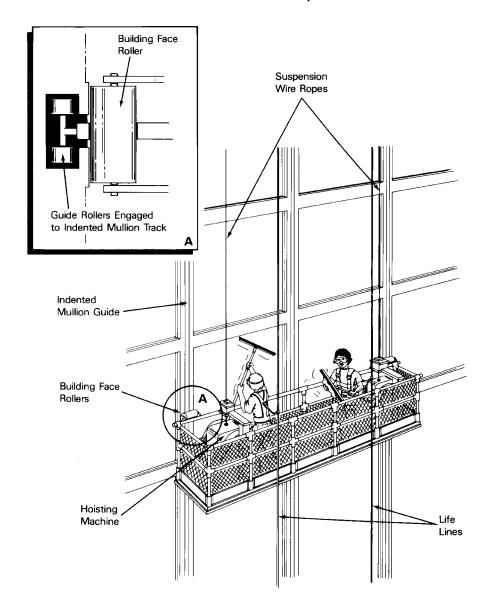
Figure 2. Typical Self-Powered Platform--Intermittent Tie-In System
