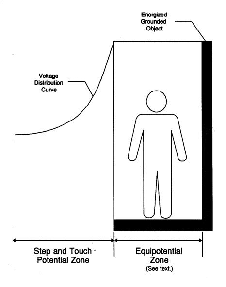
Figure 3 - Protection from Ground-Potential Gradients
